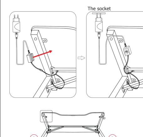
Put sticker on the control box, paste the control box at the bottom of the desktop.
