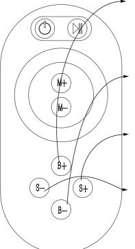
**B+**: The output signal brightness control, every time you press this button, the brightness series add 1, altogether 25 levels.
